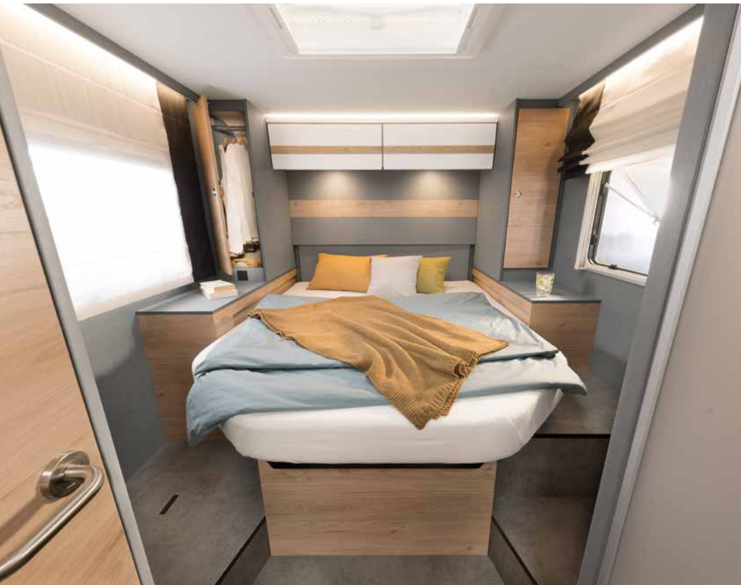
Comfortable and practical: the queen bed is height-adjustable and accessible from three sides. This means you can either have more space in the rear garage or extra headroom in the bedroom • T 7052 DBL
