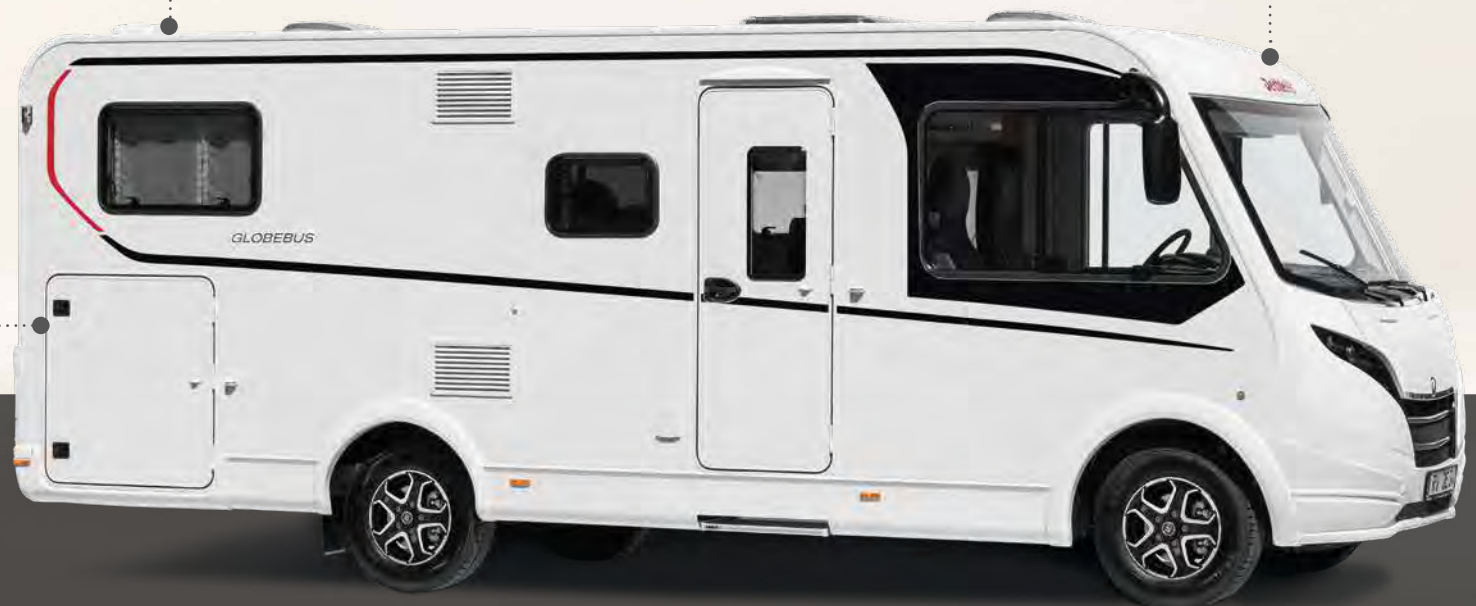
Tall rear garage with access from both sides and max. 150 kg distributed load
