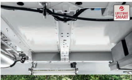
» Wood-free and rot-free Lifetime Smart floor construction (covered with GRP).
