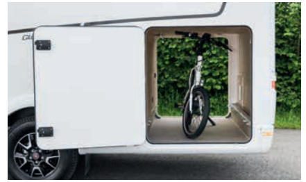
» High garage with 150 kg loading capacity. Two garage doors are standard.
