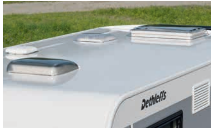
» Well-protected against hail: durable GRP roof.
