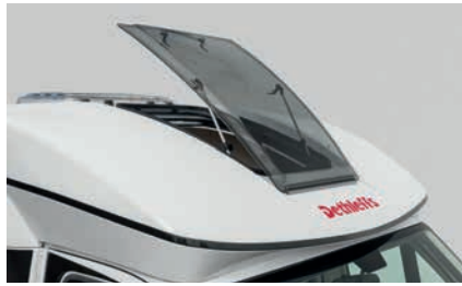
» T: Large opening skylight in T-hood.
