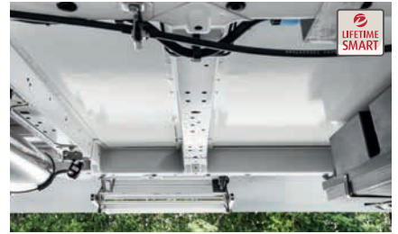
» Wood-free and rot-free Lifetime Smart floor construction (covered with GRP).
