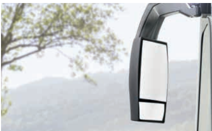
» I: Double mirror for an optimised field of view.
