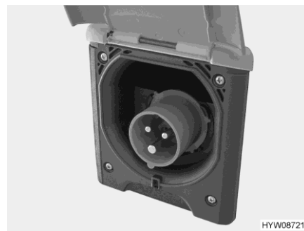
Fig. 58 230 V connection on the vehicle (CEE socket outlet)
