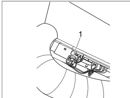
Fig. 77 Fuse under the seating group
