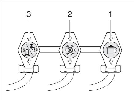
Fig. 61 Symbols for the gas isolator taps
